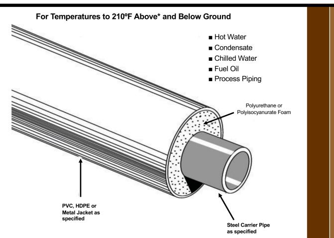
Rovanco's Steel System is designed for piping systems above or below ground suitable for inside or outside applications. High quality polyurethane foam insulation combined with a durable watertight jacket supplied in 20' or 40' random lengths, means an economical, highquality system.
