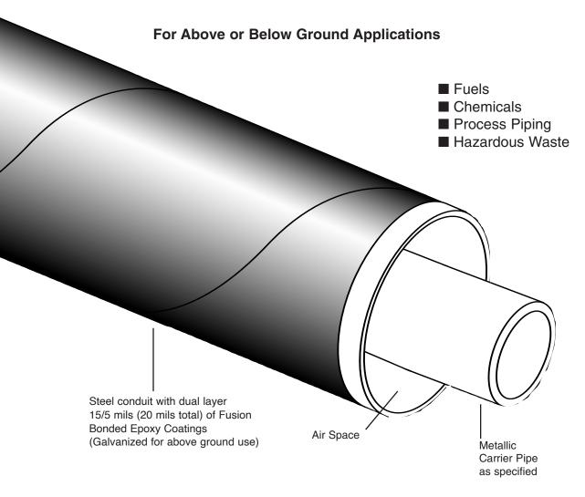
Rovanco's Containment Conduit is designed for piping systems with durable 10 gauge minimum thickness metal conduit. Supplied in 40' lengths, means an economical, high-quality system.
