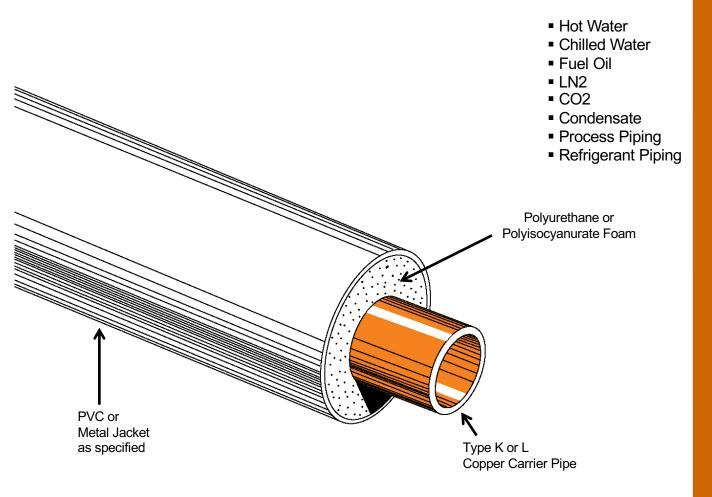
Rovanco's Copper Systems is designed for piping systems above or below ground suitable for inside or outside applications. Carrier pipe insulation is either a polyurethane or polyisocyanurate high quality foam, combined with a durable watertight jacket supplied in 20' lengths, means an economical, high-quality system.
