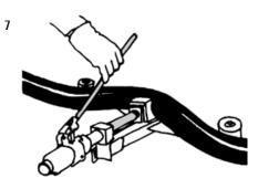
Pipes sizes up to 1 ½" can be bent by hand. When laying SECON-X $^{\circ}$  2" and bigger, it is advisable to use a bending machine, particularly if the pipes are to be laid in a building, channel or conduit.
