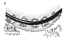
Cable rollers reduce friction and protect the pipe if it has to be laid around sharp corners. It makes work easier, particularly on stretches with a large number of curves.
