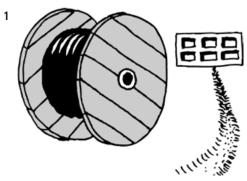
You will have received our SECON-X® Pipe in a coil or on a cable reel. Ideally, you should position the drum in such a way that the pipe can be unreeled directly from the drum.
