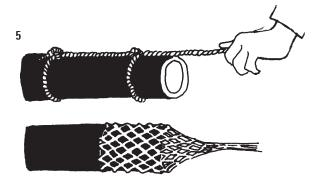
If you are working with a steel traction cable, use an end-piece made of hemp or nylon and tie an offset double knot. If there is a risk of the tied end to jam, use a cable stocking. These can be purchased from our company.
