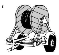
For large pipe diameters or longer sections of pipe, it is best to use a cable-laying trailer. We recommend to contact an electric cable laying company in your area.
