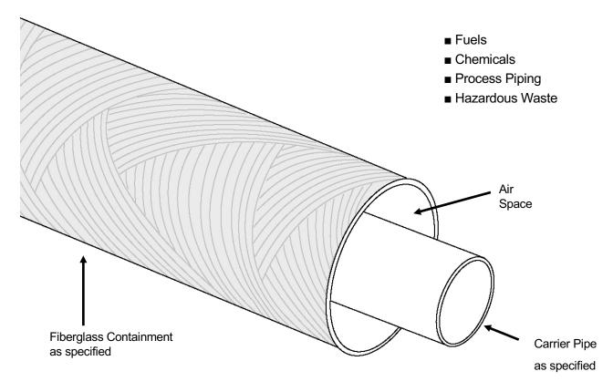
Rovanco's FRP Containment System is designed for applications of high quality with durable FRP casing. All elbows, tees, and end seals are supplied as a standard product for field fabrication.
