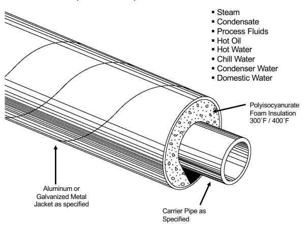
Rovanco's Hi-Temp is designed for piping systems above ground suitable for indoor or outdoor applications. 25/50 Flame/Smoke rated polyisocyanurate insulation and durable metal jacket supplied in 20' or 40' lengths, means an economical, high-quality system.
