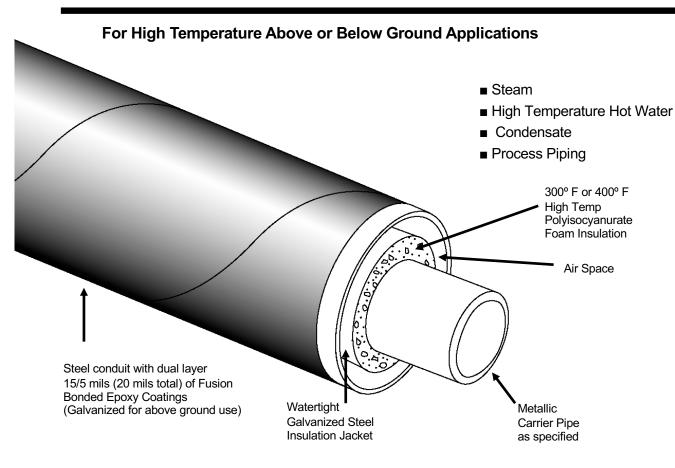
Rovanco's HTF Conduit is designed for piping systems suitable for up to 300°F or 400°F applications. insulation Polyisocyanurate with watertight galvanized jacket covering the foam insulation, and a durable 10 gauge minimum thickness steel conduit supplied in 40' lengths, means an economical, high-quality system.
