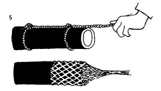
If you are working with a steel traction cable, use an end-piece made of hemp or nylon and tie an offset double knot. If there is a risk of the tied end to jam, use a cable stocking. These can be purchased from Brugg Pipesystems.
