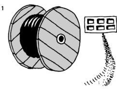
You will have received our FLEXWELL®-HL Pipe in a coil or on a cable reel. Ideally, you should position the drum in such a way that the pipe can be unreeled directly from the drum.
