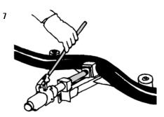
Pipes sizes up to 48/71 (1 ½") can be bent by hand. When laying FLEXWELL®-HL Pipes 60/83 (2") and bigger, it is advisable to use a bending machine, particularly if the pipes are to be laid in a building, channel or conduit.
