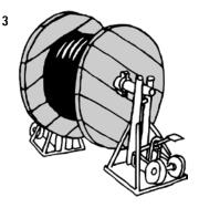
Hydraulic jacks simplify the work. These are worth purchasing if you are frequently involved in laying FLEXWELL®-HL Pipes.
