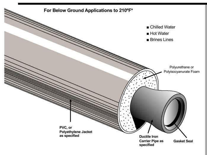
Rovanco's Ductile Iron System is designed for underground applications of chilled water or hot water. Carrier pipe insulation is either a polyurethane or polyisocyanurate high quality foam, combined with a durable plastic jacket supplied in 20' random lengths, means an economical, high-quality system.
