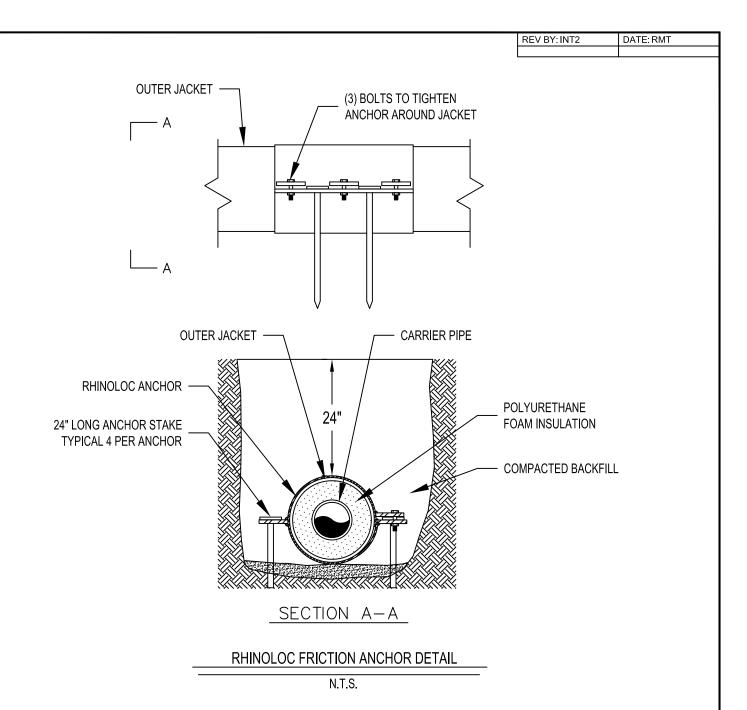
FOR SOME PRE-INSULATED PIPING SYSTEMS, THE EXPANSION FORCES ARE SUCH THAT THE ANCHOR STAKES AND COMPACTED BACKFILL ARE ADEQUATE TO ANCHOR THE PIPING SYSTEM. IN THESE INSTANCES, A CONCRETE ANCHOR IS NOT REQUIRED.
