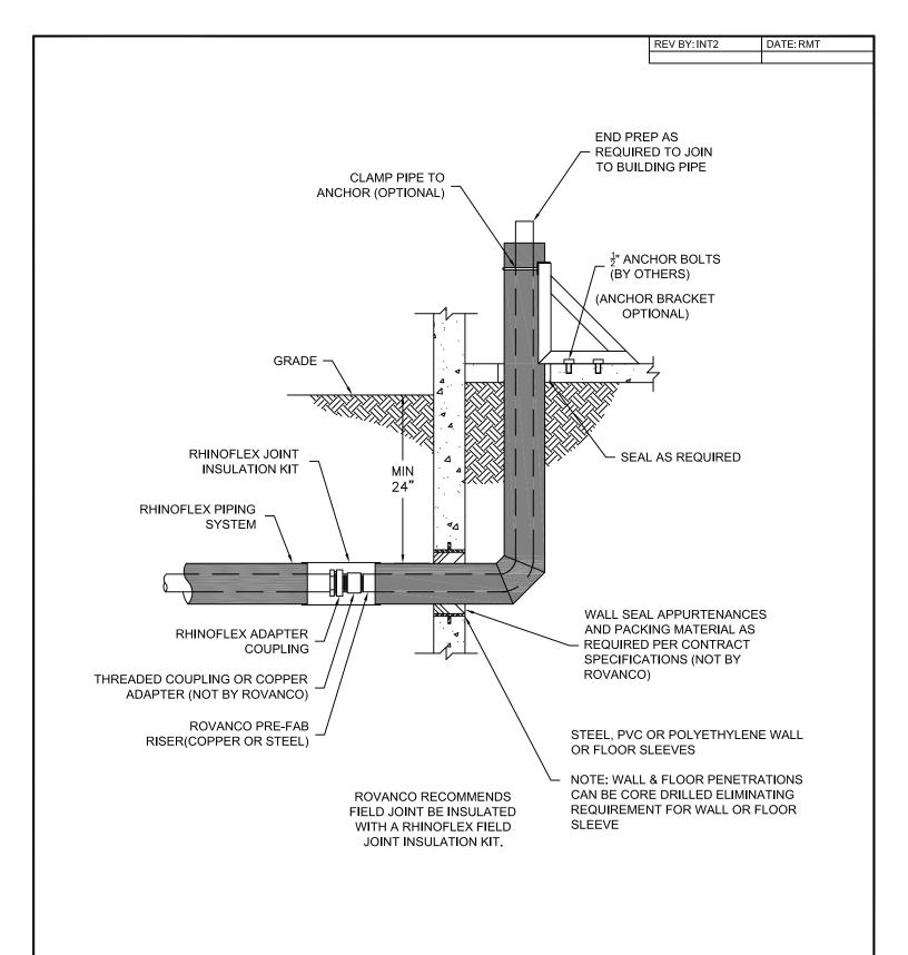
SLAB ON GRADE WHEN VERTICAL ENTRY CLOSE TO EXTERIOR WALL IS REQUIRED
