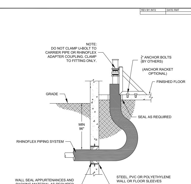
WALL SEAL APPURTENANCES AND PACKING MATERIAL AS REQUIRED PER CONTRACT SPECIFICATIONS (NOT BY ROVANCO)
