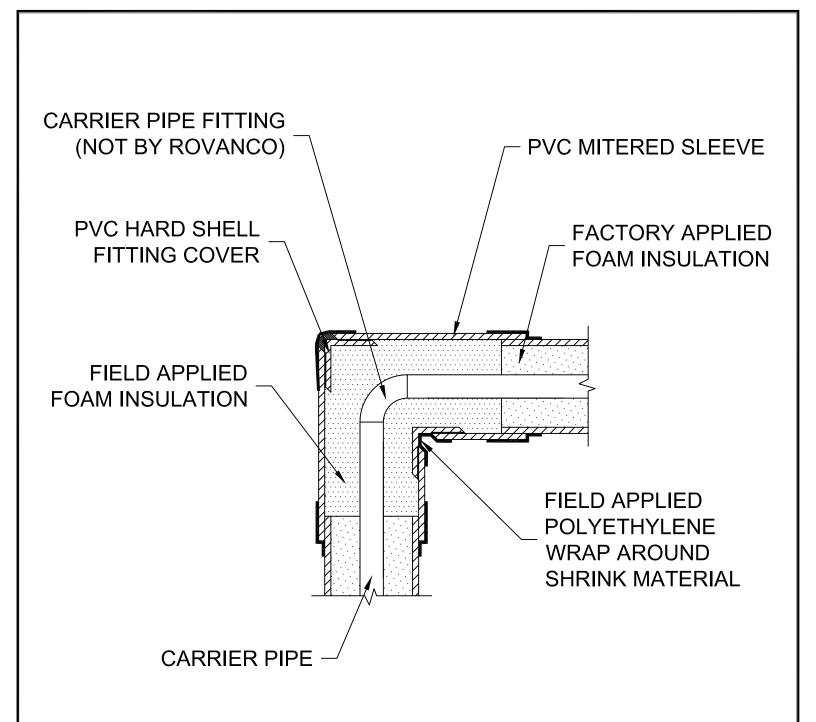
MITERED HARD SHELL FITTING COVER DETAIL
