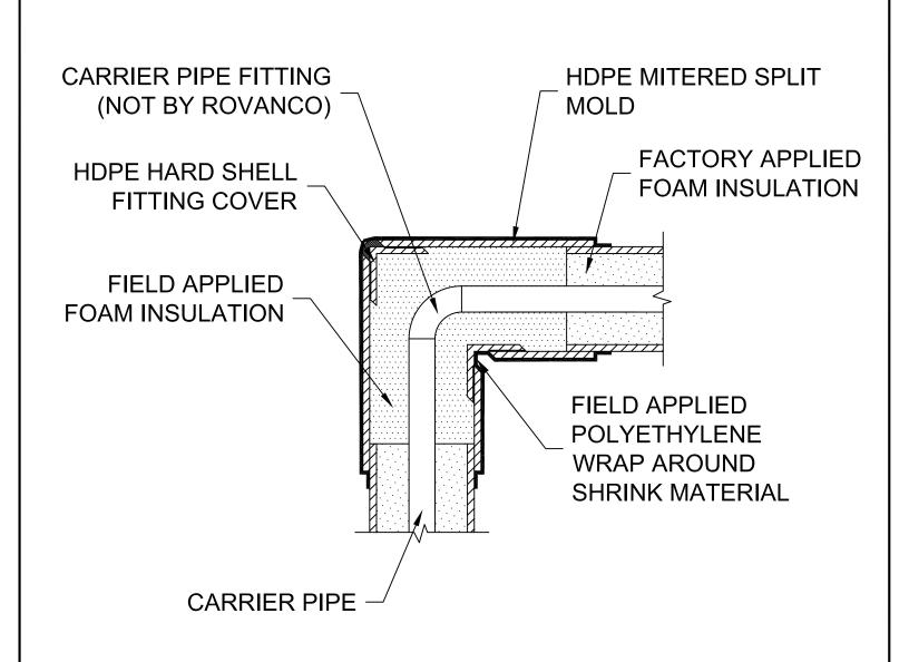
MITERED HARD SHELL FITTING COVER DETAIL N.T.S.
