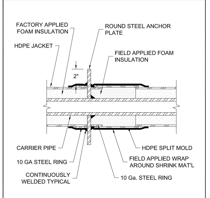
FIELD APPLIED STEEL ANCHOR DETAIL N.T.S.
