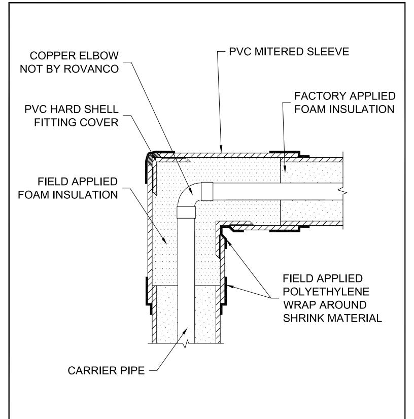
MITERED HARD SHELL FITTTING COVER DETAIL N.T.S.
