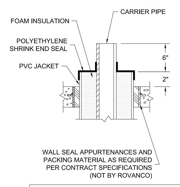
ALL OF OUR DIMENSIONS ARE TAKEN FROM END OF CARRIER PIPE AT WALL PENETRATIONS.
