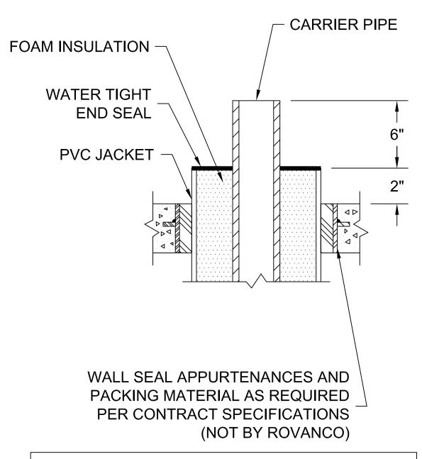
ALL OF OUR DIMENSIONS ARE TAKEN FROM END OF CARRIER PIPE AT WALL PENETRATIONS.
