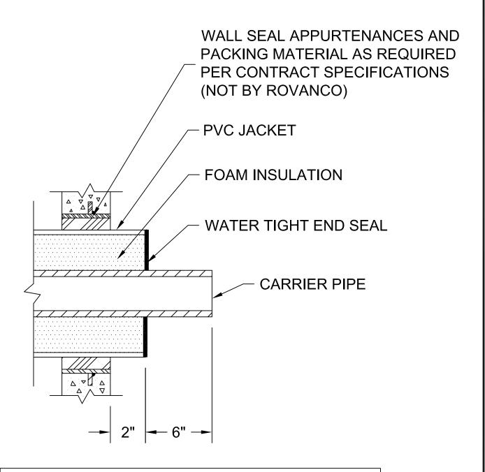
ALL OF OUR DIMENSIONS ARE TAKEN FROM END OF CARRIER PIPE AT WALL PENETRATIONS.
