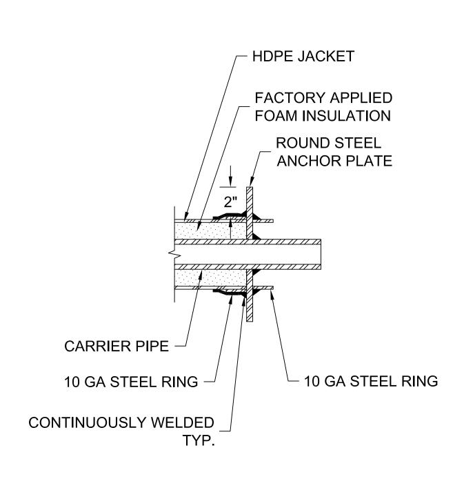
**FACTORY APPLIED ANCHOR DETAIL** N.T.S.
