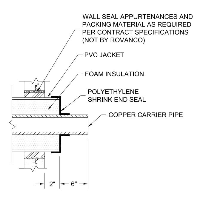
ALL OF OUR DIMENSIONS ARE TAKEN FROM END OF CARRIER PIPE AT WALL PENETRATIONS.
