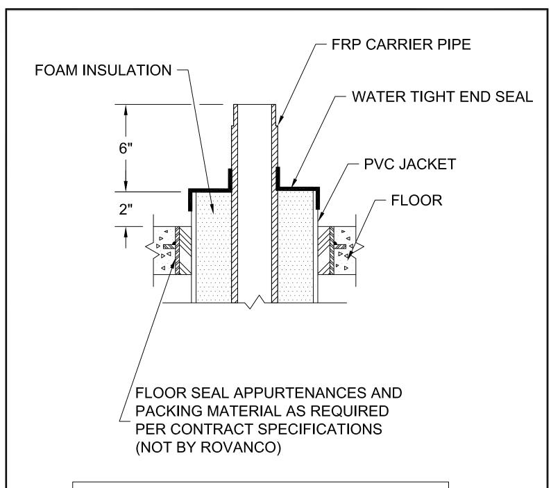
ALL OF OUR DIMENSIONS ARE TAKEN FROM END OF CARRIER PIPE AT WALL PENETRATIONS.
