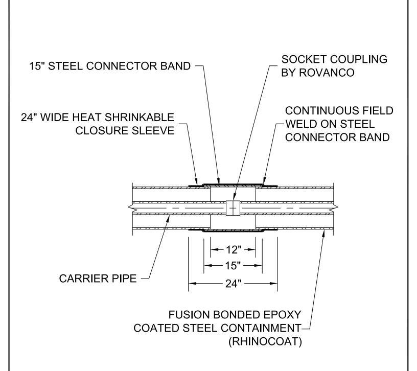
NOTE: FOR 1½" AND SMALLER STEEL CARRIER PIPE.
