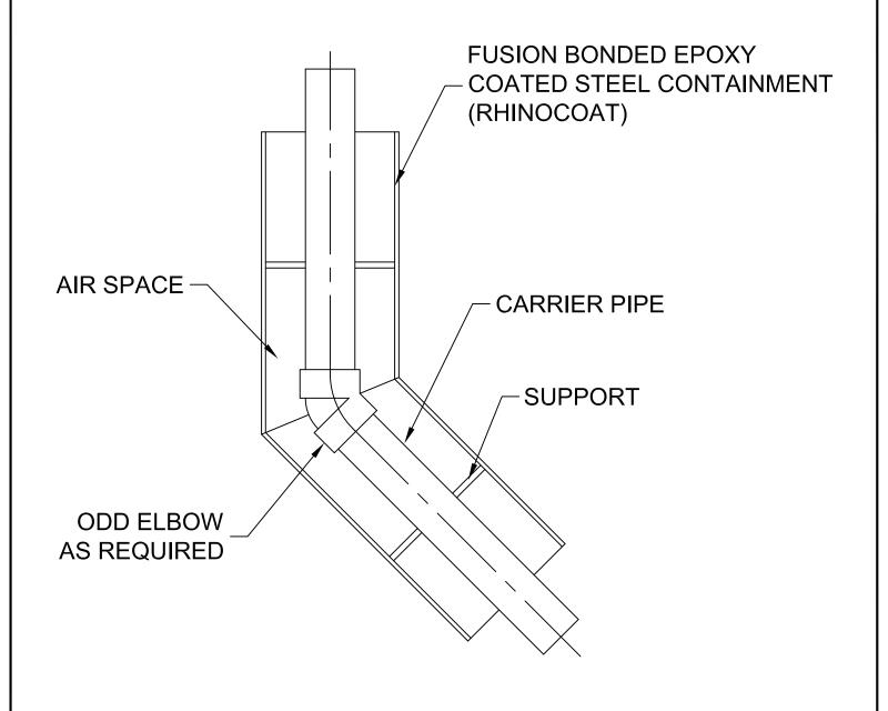
STEEL CONTAINMENT ODD ELBOW DETAIL N.T.S.
