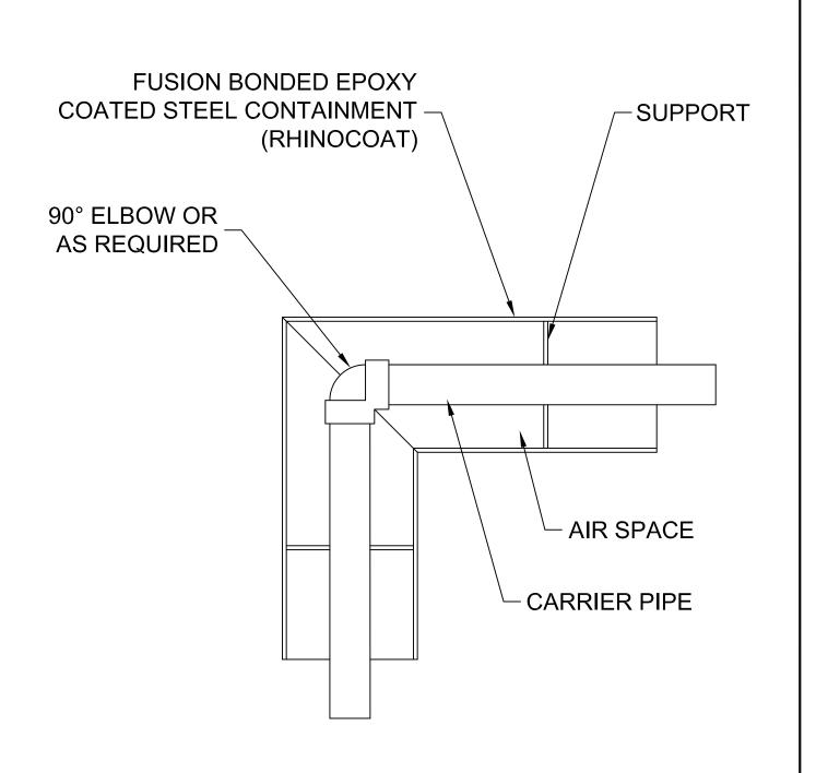
STEEL CONTAINMENT ELBOW DETAIL N.T.S.
