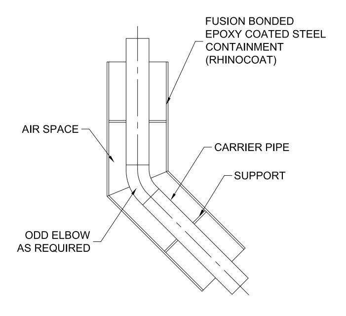
STEEL CONTAINMENT ODD ELBOW DETAIL N.T.S.
