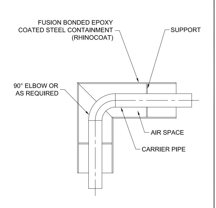
STEEL CONTAINMENT ELBOW DETAIL N.T.S.
