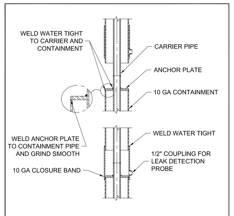
CONTAINMENT ANCHOR LEAK DETECTION PORT
