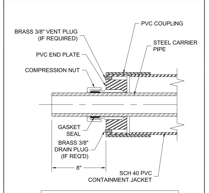
ALL OF OUR DIMENSIONS ARE TAKEN FROM END OF CARRIER PIPE AT WALL PENETRATIONS.
