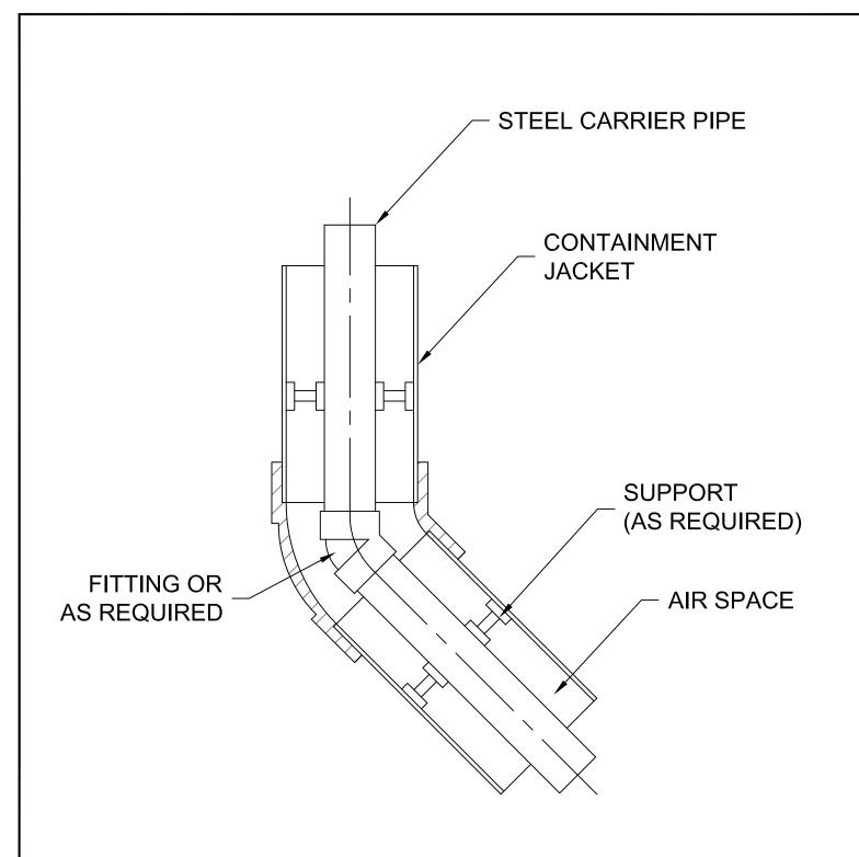
CONTAINMENT ODD ELBOW DETAIL
