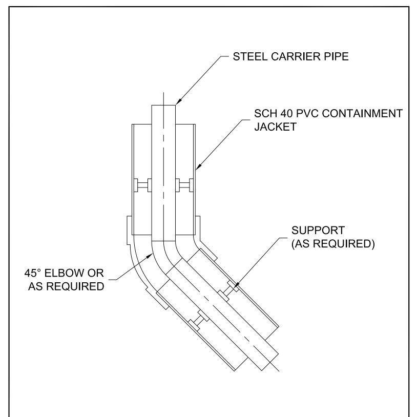
CONTAINMENT 45° ELBOW DETAIL N.T.S.
