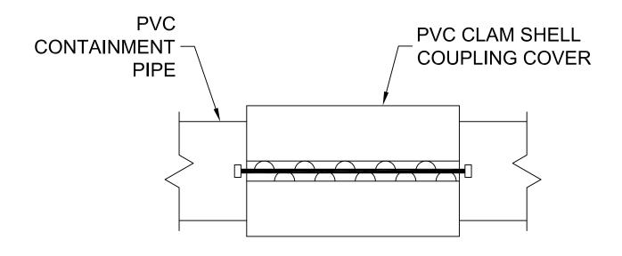
1 PVC CONTAINMENT JOINT DETAIL N.T.S.
