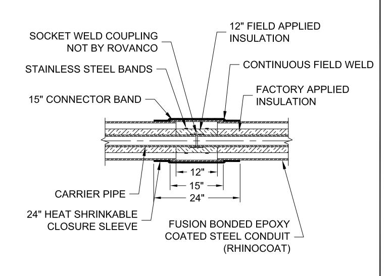
NOTE: FOR 1½" AND SMALLER STEEL CARRIER PIPE.
