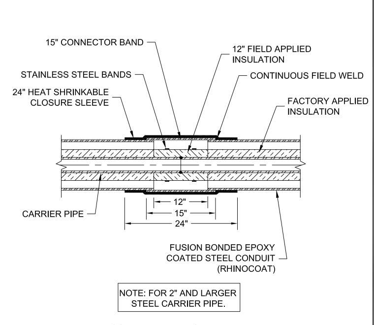
CONDUIT FIELD JOINT DETAIL
