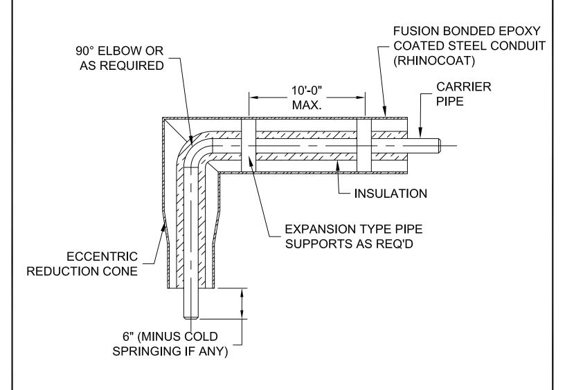
CONDUIT OVERSIZED ELBOW DETAIL
